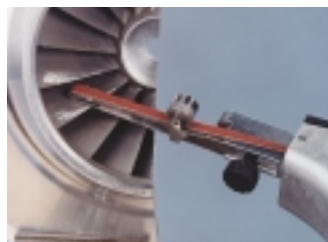
Rework turbine blades.
