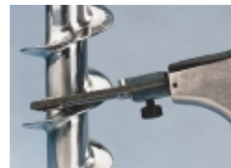
Clean and finish using Scotch-Brite® abrasive belts.
